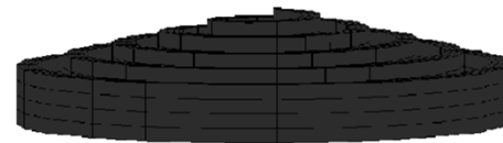
c) 12 Degree- Tapered Coil
